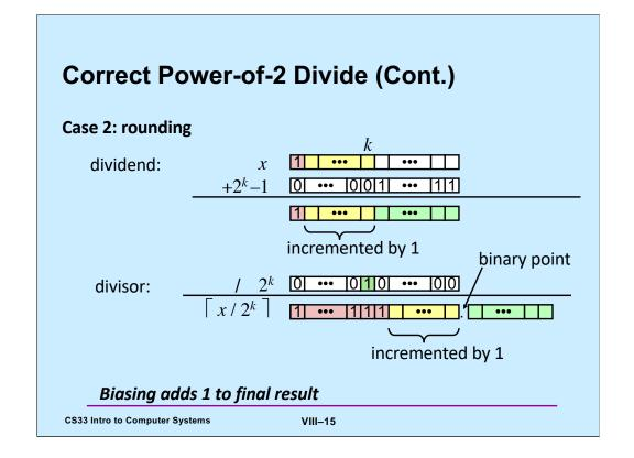
If any of the least-significant k bits are one, then adding the bias to them causes a carry of one to the bits to their left. Thus, after shifting, the number that's represented by the remaining bits is one greater (less negative) than it would have been if the bias had not been added.
