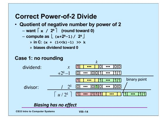
If the least-significant k bits are all zeroes, then adding in the bias and shifting right by k bits eliminates any effect of adding the bias.
