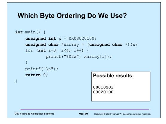
This code prints out the value of x, one byte at a time, starting with the byte at the lowest address (little end). On x86-based and m1-based (and presumably m2-based) computers, it will print:
