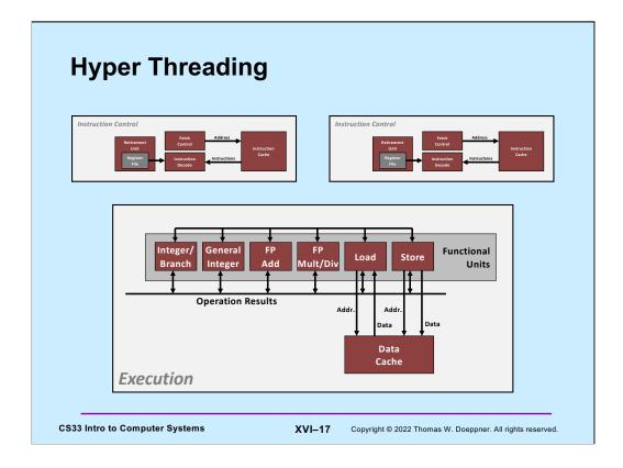
One way of improving the utilization of the functional units of a processor is hyperthreading. The processor supports multiple instruction streams ("hyper threads"), each with its own instruction control. But all the instruction streams share the one set of functional units.
