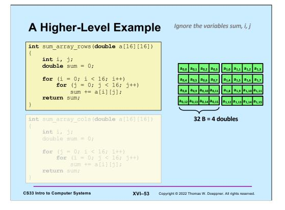
The cache still holds two rows of the matrix, but each row may go into one of two different cache lines. In the slide, the first row goes into the first lines of the cache sets, the second row goes into the second lines of the cache sets.
