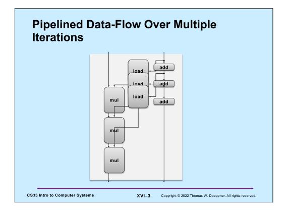
The loads depend only on the computation of the array index, which is quickly done by addition units. Thus, the loads can be pipelined.
