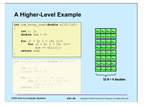
Note that the cache holds two rows of the matrix; each cache block holds four doubles. When a[0][0] is read, so are a[0][1] through a[0][3]. Thus, after one cache miss, we get three hits.
