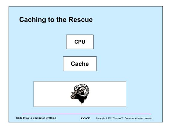
Sitting between the processor and RAM are one or more caches. (They actually are on the chip along with the processor.) Recently accessed items by the processor reside in the cache, where they are much more quickly accessed than directly from memory. The processor does a certain amount of pre-fetching to get things from RAM before they are needed. This involves a certain amount of guesswork, but works reasonably well, given well behaved programs.
