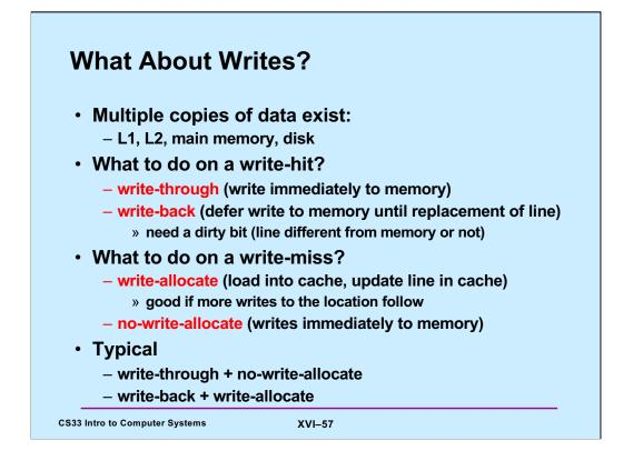
Most current processors use the write-back/write-allocate approach. This causes some (surmountable) difficulties for multi-core processors that have a separate cache for each core.
