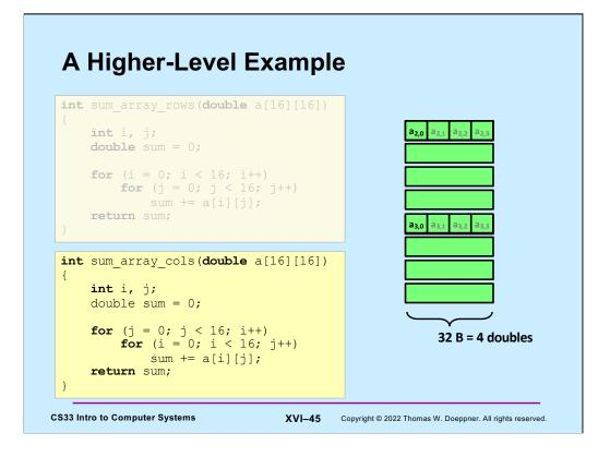
For each reference to an element of the matrix, its entire row is brought into the cache, even though the rest of the row is not immediately used.
