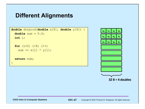
However, if the two arrays start in different cache sets, then the loop executes quickly — there is a cache miss on just every fourth access to each array.
