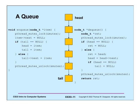
Here we have **enqueue** and **dequeue** functions that can be called by multiple threads to add and remove items from a queue. We employ a single mutex to make certain that at most one thread is performing a queue operation at a time. This could result in a bottleneck if there are lots of threads calling both of the functions. Thus, we might seek a solution that employs separate mutexes for callers to enqueue and for callers to dequeue.
