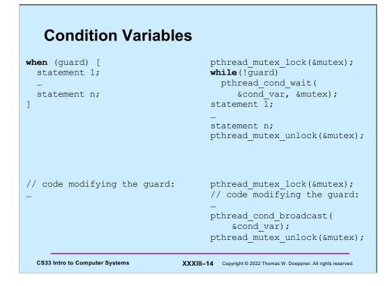
**Condition variables** are another means for synchronization in POSIX; they represent queues of threads waiting to be woken by other threads and can be used to implement guarded commands, as shown in the slide. Though they are rather complicated at first glance, they are even more complicated when you really get into them.
