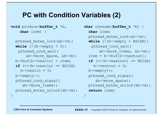
Here we have the remaining code of our solution. A producer, if there is at least one empty slot, fills the one at location **nextin**, increments **nextin** (taking wraparound into account), calls **pthread\_cond\_signal** to notify any waiting consumers that there is now an occupied slot in the buffer, and releases the mutex. If there are no empty slots in the buffer, the producer calls **pthread\_cond\_wait** to wait for one.
