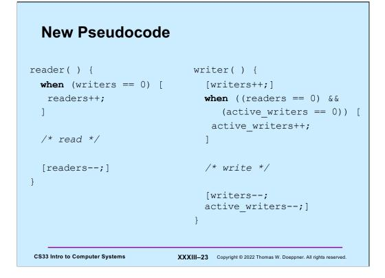
It turns out that our solution to the readers-writers problem has a flaw: writers may have to wait indefinitely before being allowed to write. This is because as long as there is a reader reading, further readers are allowed in, and writers are prevented from writing.
