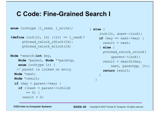
And here is the fine-grained search function. Note that its last argument indicates whether it's called by a thread that's only searching the tree, or by a thread that intends to modify the tree. Note also that the routine assumes that the parent node is locked by the caller (and that the key being searched for is not in the parent node).
