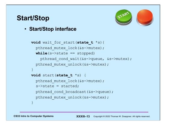
This code actually works; it uses a POSIX threads construct known as the **condition variable**. The thread in **wait\_for\_start** first locks the mutex, then checks the state. If it's stopped, it calls **pthread\_cond\_wait**, which, all at once, puts the calling thread to sleep, enqueues it on the queue (known as a **condition variable**), and unlocks the mutex.
