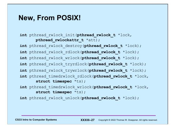
With POSIX 1003.1j support for readers-writers locks was finally introduced. The almost complete API is shown in the slide (what's missing are the operations on attributes). As might be expected, readers-writers locks can be statically initialized with the constant PTHREAD\_RWLOCK\_INITIALIZER. The "timedrwlock" routines allow one to wait until the lock is available or a time-limit is exceeded, whichever comes first.
