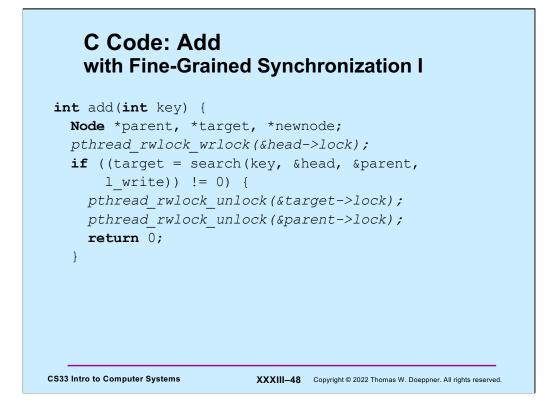
Here is the add routine modified for fine-grained synchronization.
