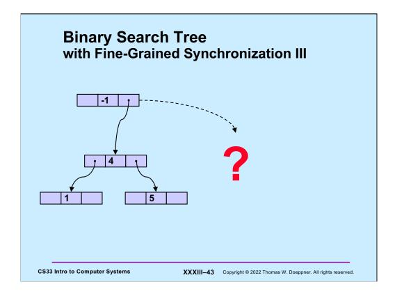
This approach could lead to trouble if after we obtain a pointer to a child and unlock a node, some other thread deletes the child (and other nodes).
