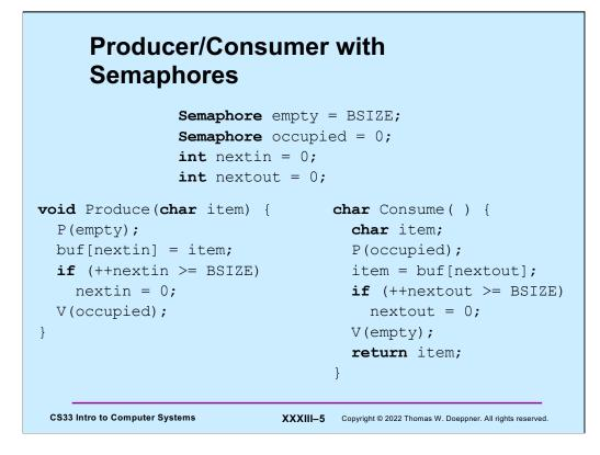
Here's a solution for the producer/consumer problem using semaphores — note that it works only with a single producer and a single consumer, though it can be generalized to work with multiple producers and consumers.
