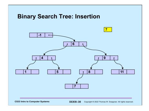
To add a new node to the tree, say one whose key will be 7, we start at the head and trace our way down the tree, comparing the new key with the keys of tree nodes, following left or right child pointers as appropriate. A new node is always inserted as a leaf.
