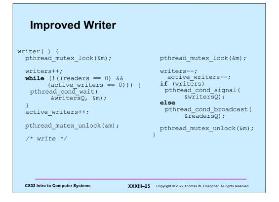
Here's the POSIX version of the writer code. Note the use of **pthread\_cond\_broadcast**: we use it to ensure that all currently waiting readers are released.
