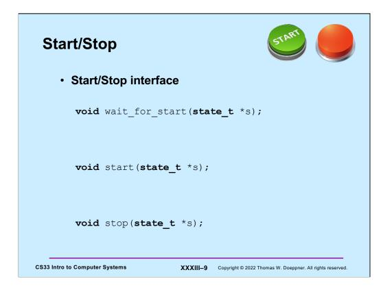
We'd like to design a "start-stop" interface. A thread calling **wait\_for\_start** waits for the **start** button to be pressed. Once it's been pressed, those waiting will be released and subsequent threads calling **wait\_for\_start** will return immediately. However, once the **stop** button is pressed, then all threads calling **wait\_for\_start** will wait until the **start** button is pressed again.
