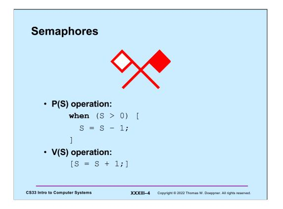
Another synchronization construct is the semaphore, designed by Edsger Dijkstra in the 1960s. A semaphore behaves as if it were a nonnegative integer, but it can be operated on only by the semaphore operations. Dijkstra defined two of these: P (for **prolagen**, a made-up word derived from **proberen te verlagen**, which means "try to decrease" in Dutch) and V (for **verhogen**, "increase" in Dutch). Their semantics are shown in the slide.
