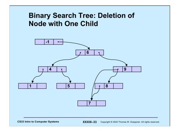
Deleting an interior node that has just one child is almost as easy. The child pointer from its parent is changed to point to the node's child, and then the node is deleted.
