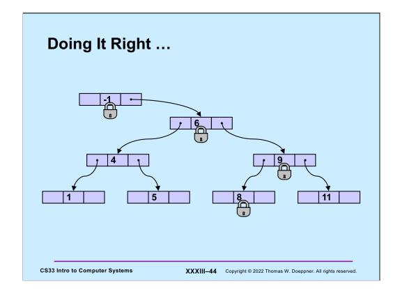
To avoid such problems, once we get a pointer to a child, we should lock the child's rw lock, and then unlock the parent's rw lock. This prevents other threads from deleting the child while we are using it.
