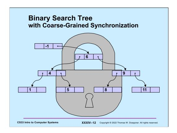
An easy way to allow multiple threads to manipulate the search tree concurrently is to employ what's known as **coarse-grained synchronization**: we associate a readers-writers lock with the entire tree. A thread that is just searching the tree for a value should take a read lock. A thread attempting to modify the tree, either adding or deleting a node, should take a write lock.
