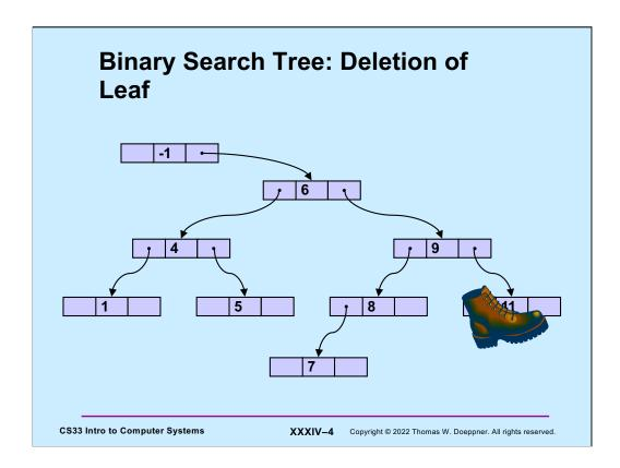
Deleting a leaf node is easy — it's simply removed and the child pointer from its parent is set to null.
