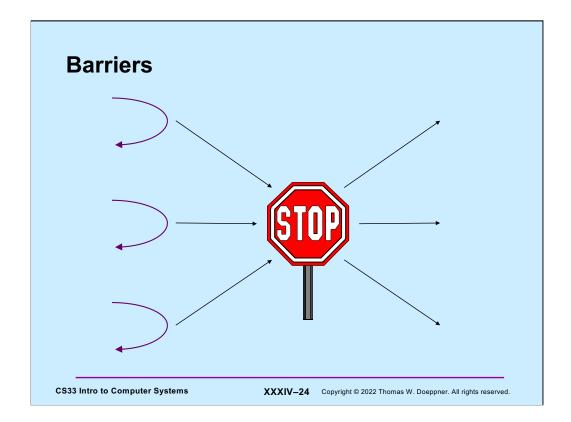
A **barrier** is a conceptually simple and very useful synchronization construct. A barrier is established for some predetermined number of threads; threads call the barrier's **wait** routine to enter it; no thread may exit the barrier until all threads have entered it.
